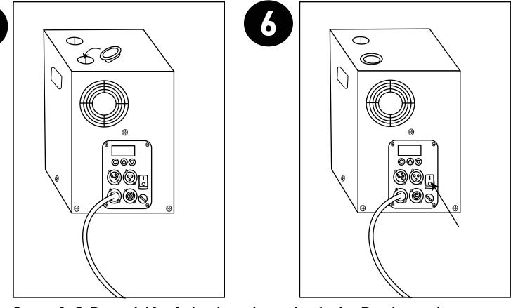
**Step 4-6** Pour 1/4 of the bag into the hole. Replace the cover and turn on the power switch.
