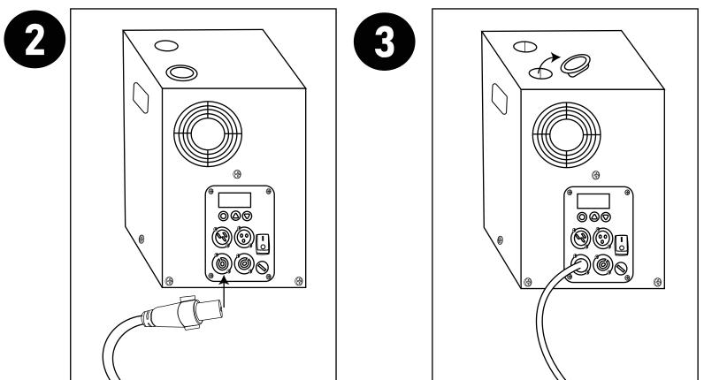
**Step 1-3** Unbox the Cold Spark and connect the power cable. Next, remove the top cover. This is where the Cold Spark powder will be inserted.
