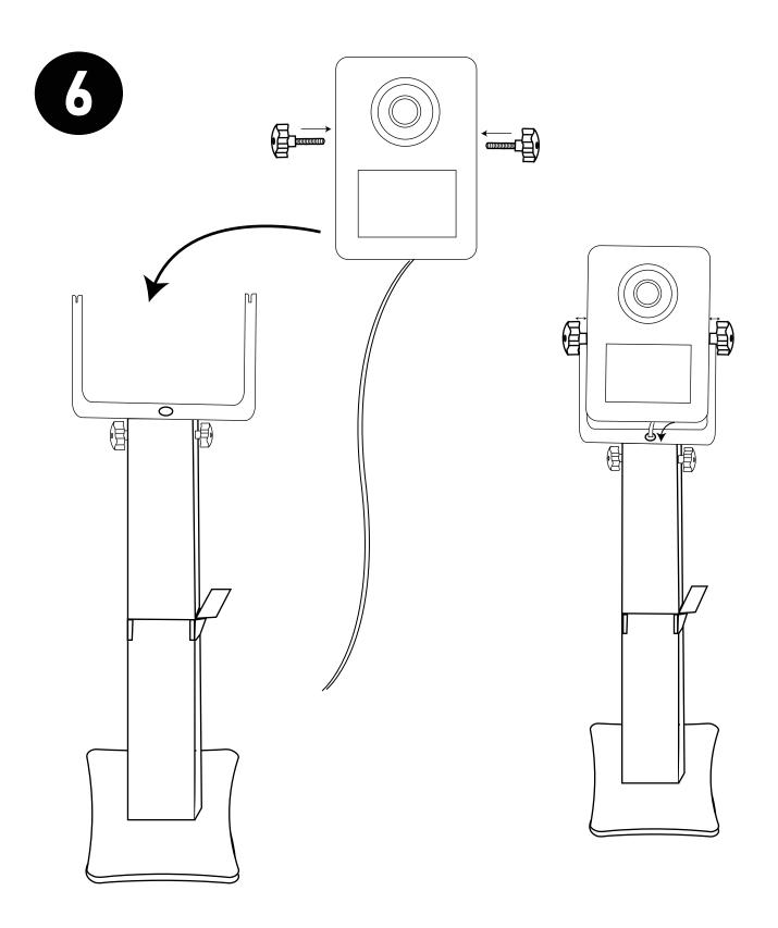
Step 6: Insert two larger knobs both side of LED and tighten with the upper stand.
