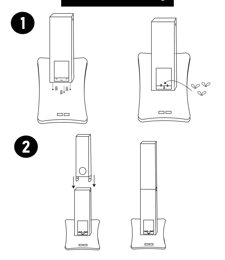
Step 1-2: Align both upright stands to the base. The holes should face the back.
