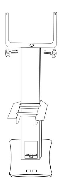
Step 5: Insert the yolk to the upright stand and tighten with the small star knobs.
