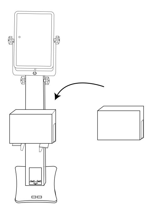
Step 7: (Optional) If you purchased the printer cover, place it on top of the printer after connecting the printer cables to the photo booth.
