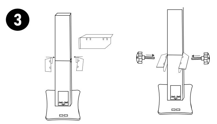
Step 3: (Optional) If you purchased the printer shelf, attach the side extensions before inserting the small star knobs.
